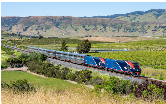
Amtrak has continued to deploy new, cleaner and faster ALC-42 diesel locomotives for Long Distance trains, including the Coast Starlight® shown above.
