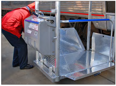
Figure 11-3 – Lowering Ground Ramp
