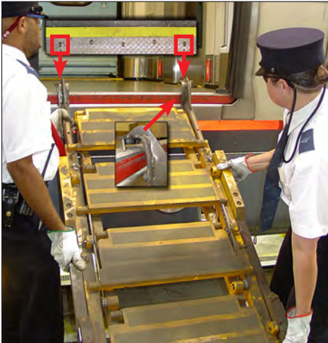
Figure 1-14 – Secure folding stairs to car body
