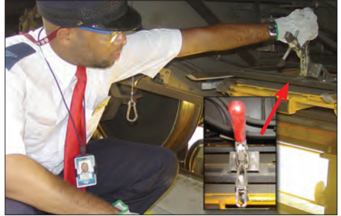
Figure 1-13 – Release folding stairs hold-down clamp
