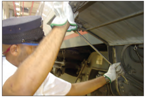
Figure 1-11 – Secure the door safety bar
