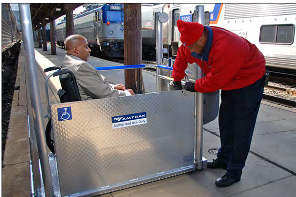
Figure 11-4 – Closing Ground Ramp
