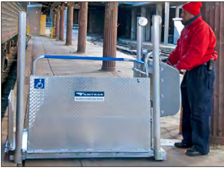
Figure 11-2 – Positioning Lift Next to Train
