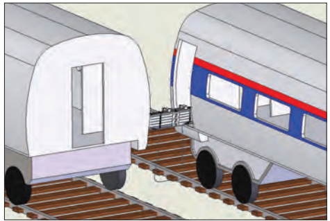
Figure 1-7 – Transfer bridge shown deployed to 2nd car in upright position. Hinged end must be fed to car #2 first with railing mounts facing up.
