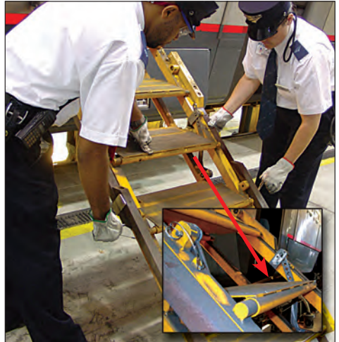
Figure 1-15 – Level stair steps
