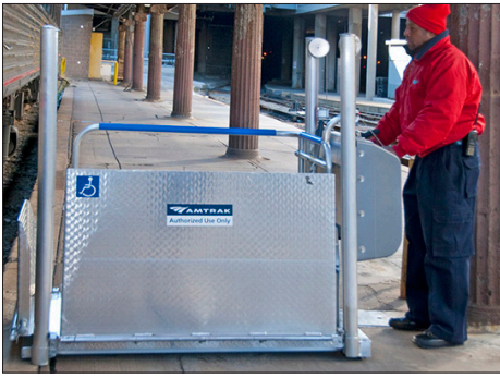
Figure 11-2 – Positioning Lift Next to Train
