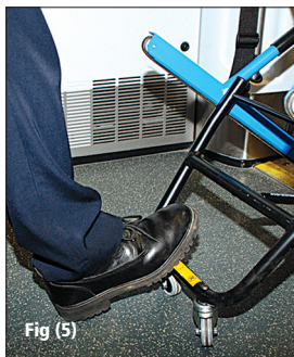
Fig (5) Align EVAC-CHAIR with top of folding stair and use foot to retract inner wheels.
