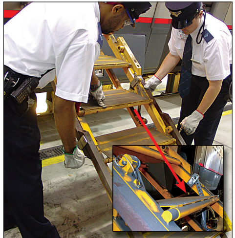
Figure 1-15 – Level stair steps
