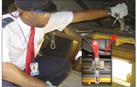
Figure 1-13 – Release folding stairs hold-down clamp
