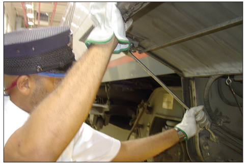
Figure 1-11 – Secure the door safety bar
