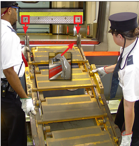
Figure 1-14 – Secure folding stairs to car body
