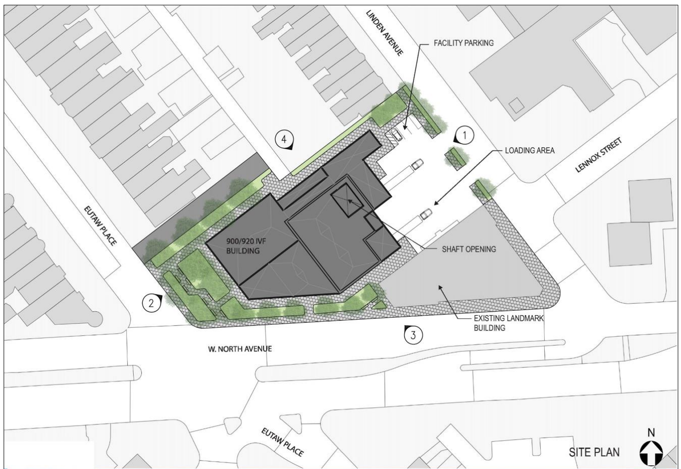
Figure 19: Representative site layout, intermediate ventilation facility. The building labeled as “existing landmark building” is 900-940 W. North Avenue, a row of one-story commercial buildings that are contributing to the Reservoir Hill Historic District, but considered of low historic value. Numbered arrows 1 – 4 refer to the direction of view of the four renderings showing representative building elevations.
