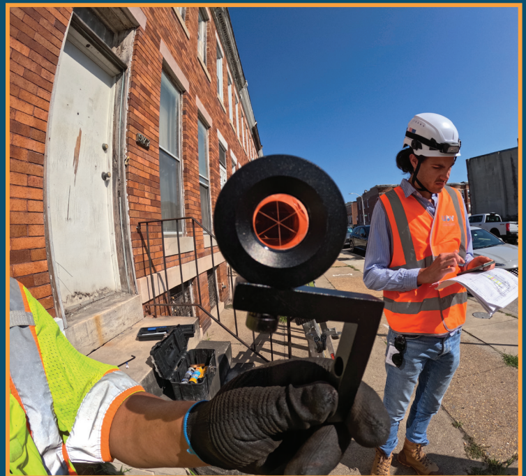
Tilt monitoring prism
